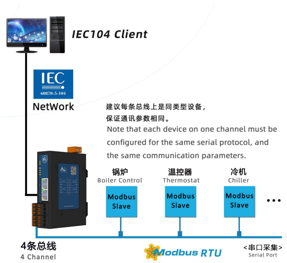
场景2: 集成串口协议 (以Modbus RTU为例) 到IEC104 Client Application-2: Connecting Modbus RTU to IEC104 Client
