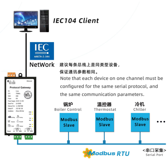
场景2: 集成串口协议 (以Modbus RTU为例) 到IEC104 Client Application-2: Connecting Modbus RTU to IEC104 Client
